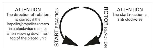
In large pumps, the direction of rotation can also be recognized by looking through the discharge outlet into the pump chamber.
