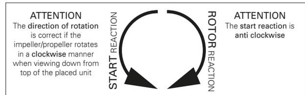
For large pumps, the direction of rotation can also be detected by looking through the pressure outlets into the pumping chamber. Here the impeller can be seen and the direction of rotation of the impeller, when discharged, can be controlled when started briefly.
